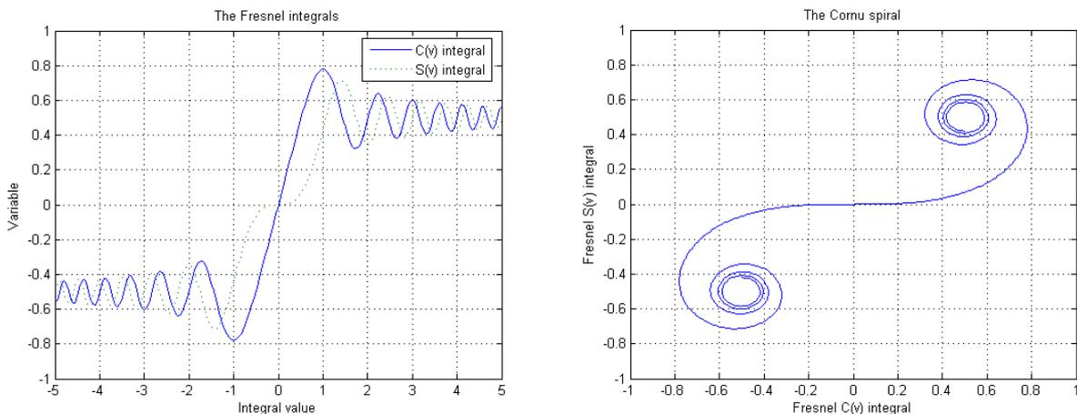
**The Fresnel cosine and sine integrals are shown to the left showing the oscillations, and the Cornu spiral is shown to the right using the cosine integral as abscise and the sine integral as ordinate.**
