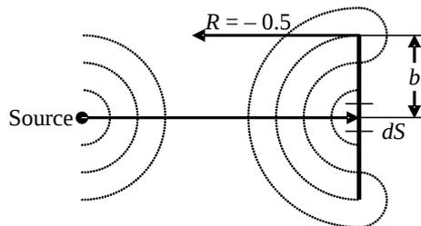
**The pressure is suddenly reduced when the wave front passes the edge leaving  $2\pi$  space and entering  $4\pi$  space. This cause reflection to occur with the reflection coefficient  $R = -0.5$ .**
