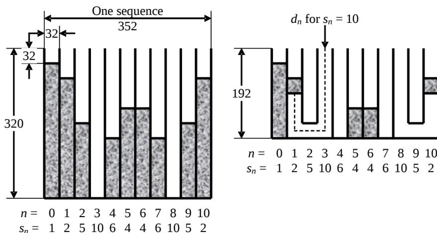
**Cross section through a QRD with three sections each with length  $N = 11$  (left) and modified for material saving and depth reduction (right). Dimensions are in millimetres.**
