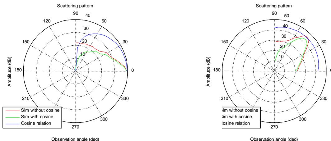
**The relation is shown for the scattered signal versus the observation angle. To the left with the source and receiver along the normal and to the right with the source and receiver offset by  $\pm 45^\circ$ , along the expected reflection paths.**
