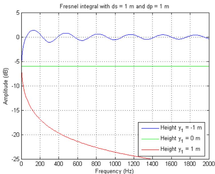
**The level of the signal at the receiver is shown for a semi-infinite baffle blocking the lower part of the propagating wave front. The direct signal is interrupted for the lower curve (red colour).**
