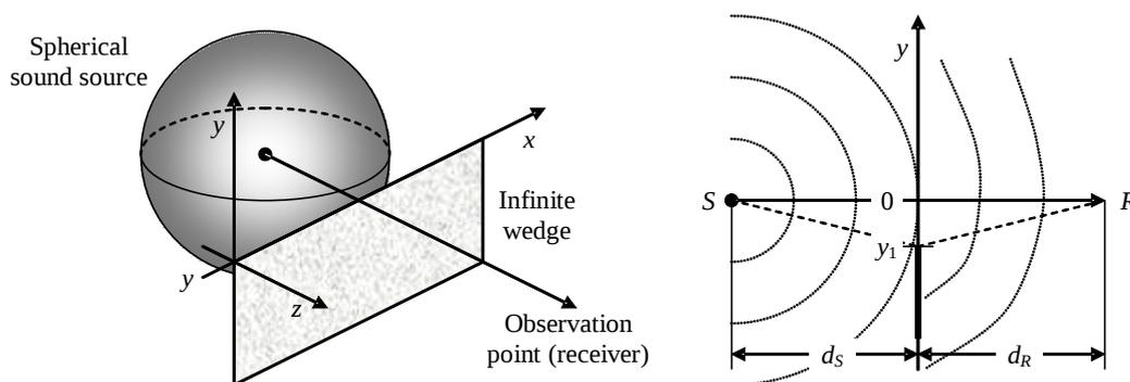
**A spherical wave front is disturbed by a semi infinite baffle and the reflections from the edge causes interference at the monitoring point.**
