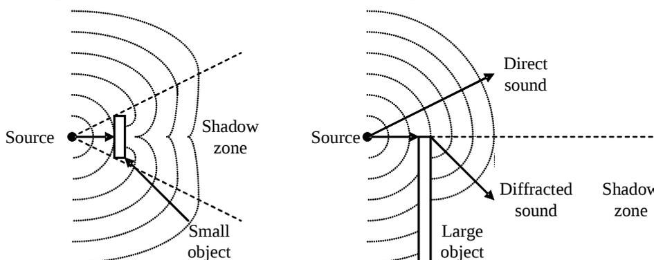
**Sound waves are not blocked by an object but are bending around the object. The sudden change in propagation impedance generates reflections from the boundary, edge diffraction and this causes interference with the direct signal at the receiving point.**
