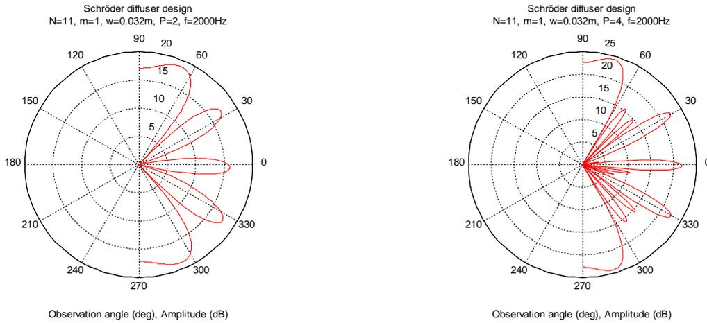
Using several periods of the diffuser results in constructive interference at 0° observation angle and side lobes. The location of the lobes is given by the diffuser width  $Nw$  as shown in section 2.4.
