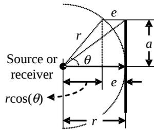
**The spherical wave form reaches the centre before the edge so the signal from the outer range is delayed with respect to the scattering from the centre of the panel.**
