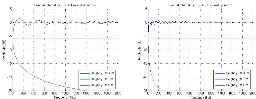
**Transfer function with source 1 m from baffle (left) or 0.1 m (right) and the observer 1 m from baffle measured at three different edge heights. The parameter  $d_p$  corresponds to  $d_r$  used within this document.**
