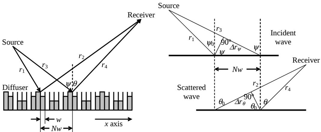
The scattering from different sections of a surface cause interference at the receiver. To the right is shown details of incident and scattered waves in order to calculate the difference in path lengths.
