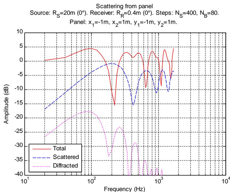
**The response of the scattered sound for the source at 20 m and the receiver 400 mm from the panel with the measure 2 m by 2 m.**
