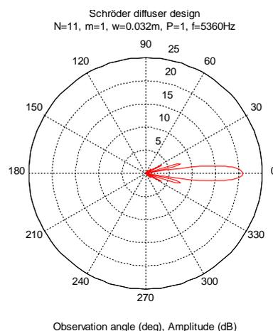
**To the left is shown the scattering pattern when operating within the intended frequency range, and to the right when operated right at the critical frequency corresponding to a plane and rigid plate.**
