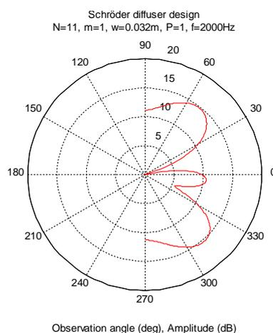
**The scattering patterns at two frequencies within the intended frequency range.**
