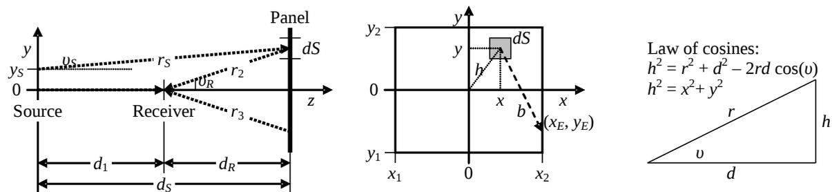
The calculation of distances uses Pythagoras and the calculation of the angle of incidence uses the cosine law.
